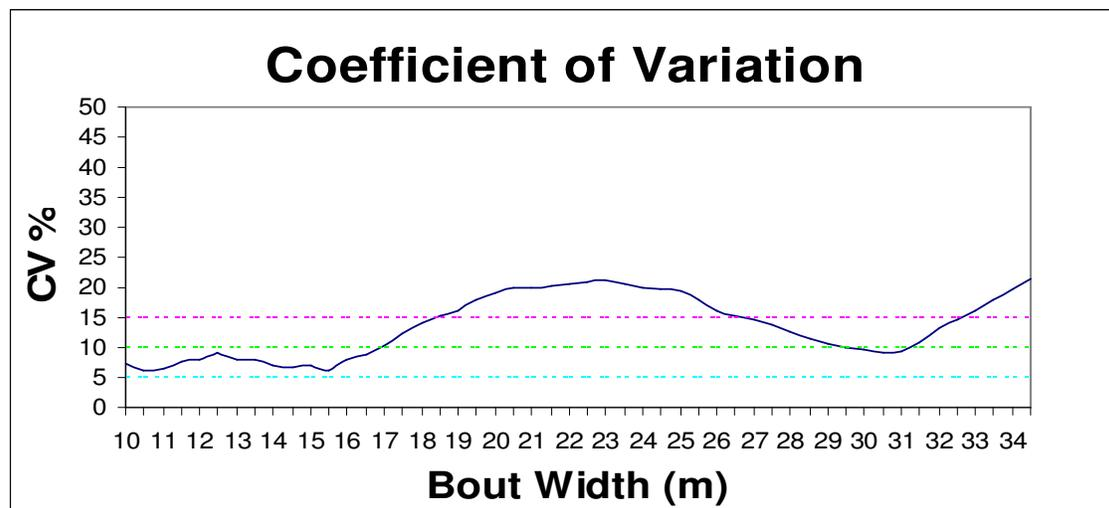
Fig 2 shows how CV% rises for a swath pattern of the shape shown in Fig 1. The higher the CV% value the poorer the overall distribution. In this example a bout width (effective swath width) of 31m as shown by the red lines will give an evenness of application of 10 (CV %) which means it is very even spreading. Under Spreadmark, the maximum permissible CV % for a nitrogen based fertiliser is a pattern test is 15%
