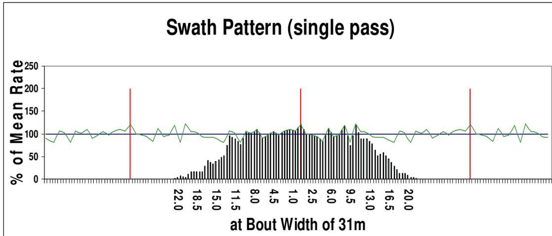
Fig 1 shows a good spread pattern of an aircraft for round and round (R&R) travel applying urea – the black vertical lines show the amount of solid particles collected in each tray. The total swath width is about 44m.
