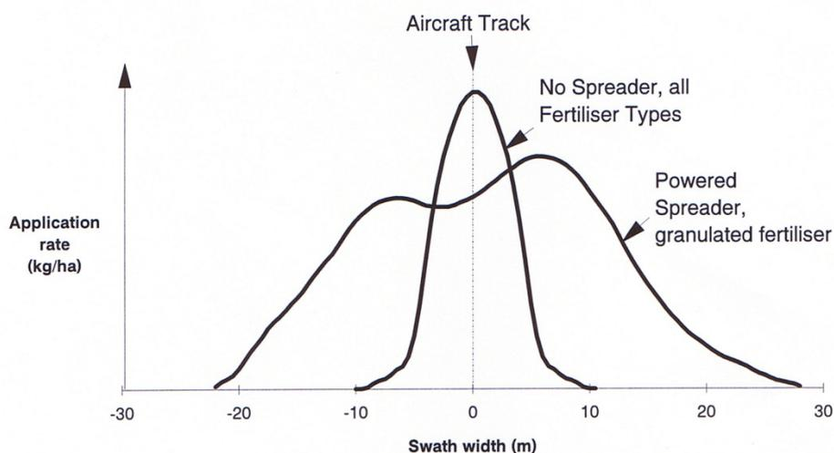
**Fig 3.2** Single pass spread pattern, helicopter bucket (spinning disc) spreader and no cross wind
