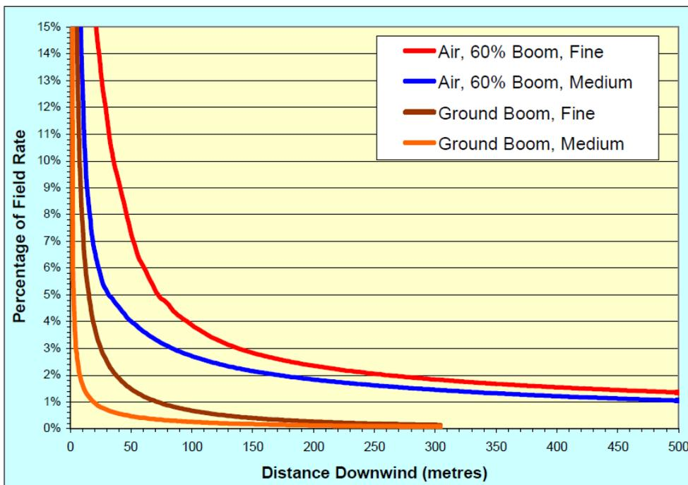
On this graph, zero on the horizontal axis represents the downwind edge of the application area. The wind is blowing from left to right. The vertical axis is scaled in percent of the intended field application rate. For example, the top curve (red) shows that approximately 4% of the intended field rate is deposited at a distance 100 metres downwind from the downwind end of the application area.
