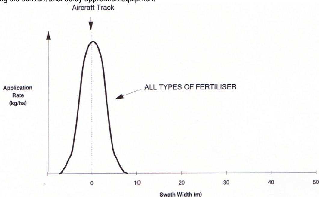
**Fig 3.1 Single pass spread pattern, no spreader and no cross wind**
