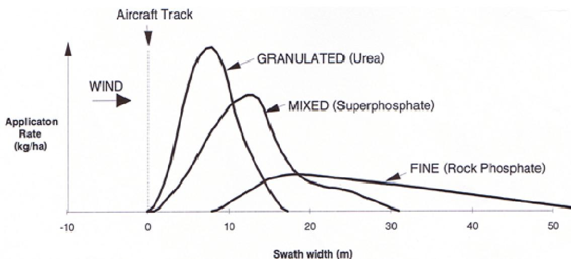
**Fig 3.4 (Crosswind effects on swath spread patterns)**
