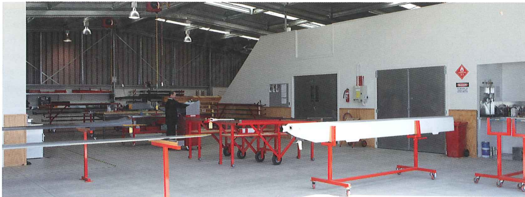
Oceania's new purpose-built rotorblade and composite repair facility. The blade in the foreground is a Bell 206.
